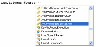
Typing a period (or pressing the tab key) displays the allowed values for the TriggerSource enumeration:
