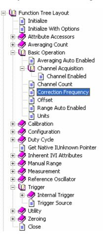
In stark contrast to the IVI-COM hierarchy, the IVI-C hierarchy gives no indication as to which attributes apply to repeated capabilities and which do not. For instance, Correction Frequency applies to a specific Channel repeated capability while Units applies to the driver as a whole. Yet, these attributes both are defined as children of the patently nondescript Basic Operation group.
