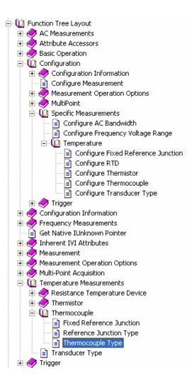
The trouble with this hierarchy is that the IVI specifications have actually defined IVI-C functions in different locations than their associated attributes. Notice that the Configure Thermocouple function is located in a completely different portion of the hierarchy than the Thermocouple Type attributes it controls.
