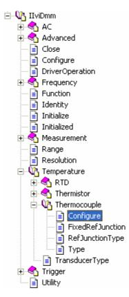
The IVI-COM hierarchy is noticeably simpler than the corresponding IVI-C hierarchy, even though they both represent the exact same functionality. For example, the Configure Thermocouple function is located in the exact same place as its associated attributes, including the Thermocouple Type attribute.
